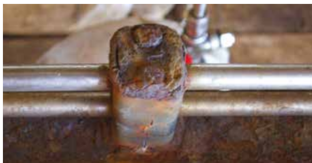
Crevice corrosion between the tube/tube trap interface.
